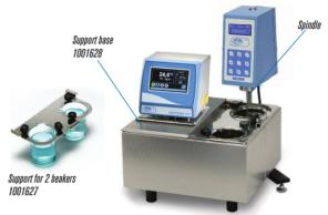
Digiterm thermostat bath with support base Part No. 1001628. 12 litre bath Part No. 6000391 and adapter kit Part No. 1001625 or 1001626 To be used with a rotary viscometer and beaker support Part No.
