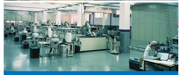
Pressurized and acclimatized room with sophisticated serial production automatisms.
