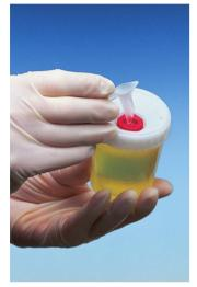
Insertion of the GALET in the AOUISEL VALVE-STOPPER.
