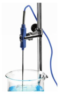
Temperature sensor Pt100. Controls the sample temperature in the digital hotplate stirrers. Immersion Probe: 4mm Ø x 130 mm long. Cable connector 150 cm long.
